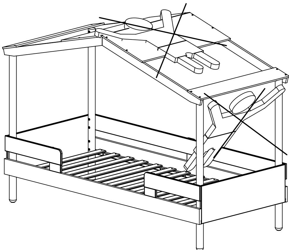
**EN:** Children can be trapped between the bed and the wall, a sloping roof, the ceiling, adjacent furnishings (e.g. cupboards) and so on. In order to avoid serious risk of injury, the distance between the upper edge and the adjacent structure must not exceed 75mm or must be greater than 230mm.
