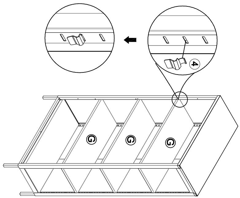
**(7) - Attach (2) & (3) to pre-assembled unit as below shown.**
