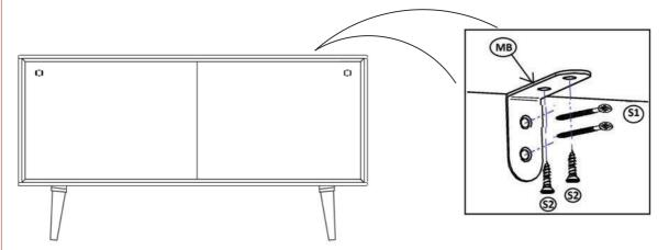
STEP 1: Using short screws, attach one of the brackets on each end of the furniture's back, on the top surface, or inside.
