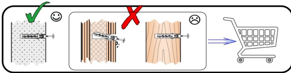
**-EN-** Before suspending or fixing furniture to the wall (in order to prevent falling over), check the type and strength of the wall. Select wall plugs and screws appropriate for the given type of the wall. In the case of doubts, contact a specialist. The installation must be performed by a competent person. **WARNING!!! If the rawlplugs with screws are attached to the product, then they are intended only for walls made of solid and homogeneous materials.**
