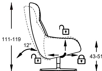
↑ Seat height adjustment: **Lighten the load on the seat** and lift the lever upwards.
