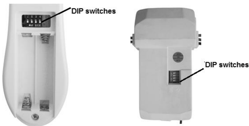
Fig. 11 Remote battery compartment
