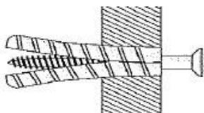
General aerated blocks should not be used to support heavy loads, use a specialist fitting in this case. For light loads, a General Purpose Plug can be used.
