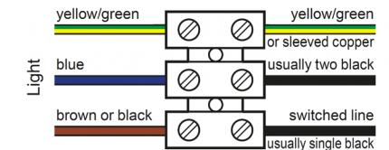
For some lamps, the protective conductor does not have to be connected to a terminal, but to a terminal on the metal parts of the lamp (screw with earth symbol ).
