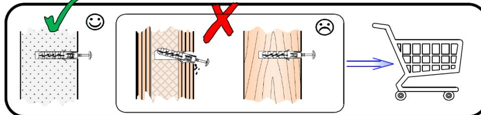
**-EN-** Before suspending or fixing furniture to the wall (in order to prevent falling over), check the type and strength of the wall. Select wall plugs and screws appropriate for the given type of the wall. In the case of doubts, contact a specialist. The installation must be performed by a competent person. **WARNING!!! If the rawplugs with screws are attached to the product, then they are intended only for walls made of solid and homogeneous materials.**
