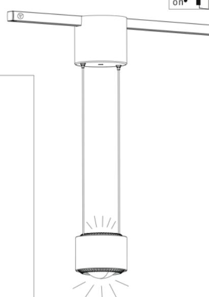
In the event that the cables between the canopy and the lamp head are twisted and not parallel to the U-Rail: To straighten the cables - run your finger and thumb along the cable.
