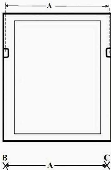
6. The mirror hanging brackets should be hung directly on these screws.
