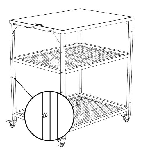
Tighten to 50% **DO NOT** over tighten bolts
