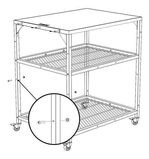
Tighten to 50% **DO NOT** over tighten bolts
