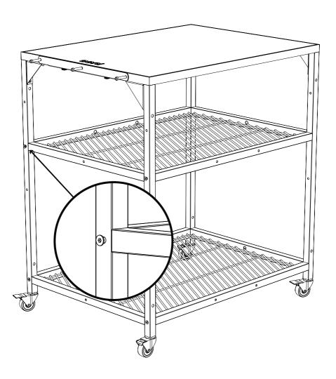
Loosen to 50% **DO NOT** over loosen bolts
